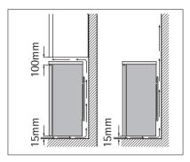
tance between the wall and the cabinet must be at least 10 mm to allow the door to open enough so that the shelves can be removed.
